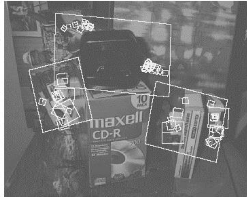
Figure 12: The training images for two objects are shown on the left. These can be recognized in a cluttered image with extensive occlusion, shown in the middle. The results of recognition are shown on the right. A parallelogram is drawn around each recognized object showing the boundaries of the original training image under the affine transformation solved for during recognition. Smaller squares indicate the keypoints that were used for recognition.
