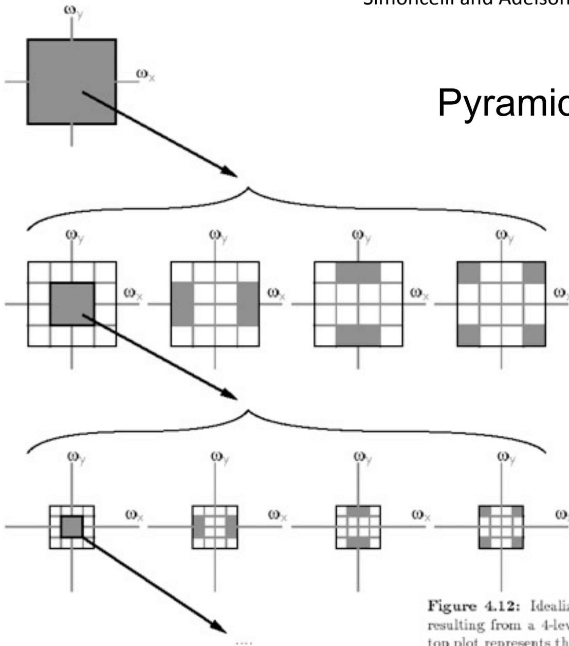
**Figure 4.12:** Idealized diagram of the partition of the frequency plane resulting from a 4-level pyramid cascade of separable 2-band filters. The top plot represents the frequency spectrum of the original image, with axes ranging from  $-\pi$  to  $\pi$ . This is divided into four subbands at the next level. On each subsequent level, the lowpass subband (outlined in bold) is subdivided further.
