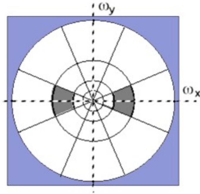
**Figure 1.** Idealized illustration of the spectral decomposition performed by a steerable pyramid with  $k = 4$ . Frequency axes range from  $-\pi$  to  $\pi$ . The basis functions are related by translations, dilations and *rotations* (except for the initial highpass subband and the final low-pass subband). For example, the shaded region corresponds to the spectral support of a single (vertically-oriented) subband.
