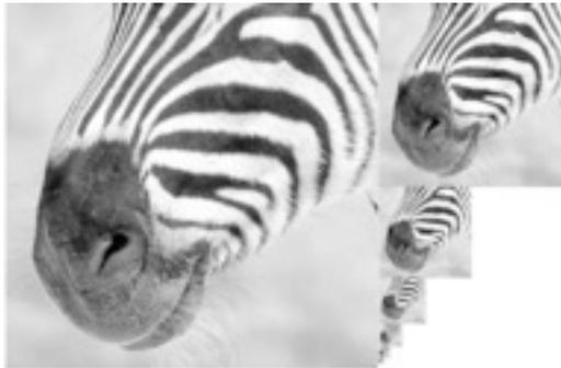
Progressively blurred and subsampled versions of the image. Adds scale invariance to fixed-size algorithms.
