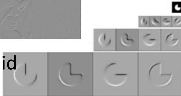
Shows components at each scale and orientation separately. Non-aliased subbands. Good for texture and feature analysis. But overcomplete and with HF residual.
