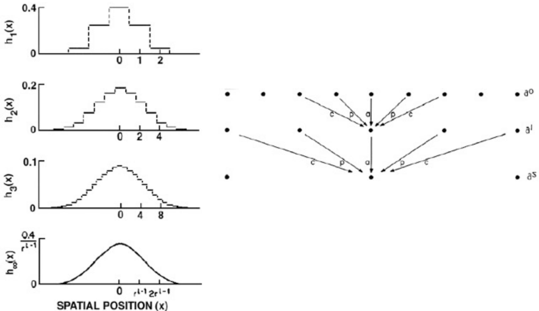
Fig. 2. The equivalent weighting functions  $h_l(x)$  for nodes in levels 1, 2, 3, and infinity of the Gaussian pyramid. Note that axis scales have been adjusted by factors of 2 to aid comparison. Here the parameter  $a$  of the generating kernel is 0.4, and the resulting equivalent weighting functions closely resemble the Gaussian probability density functions.
