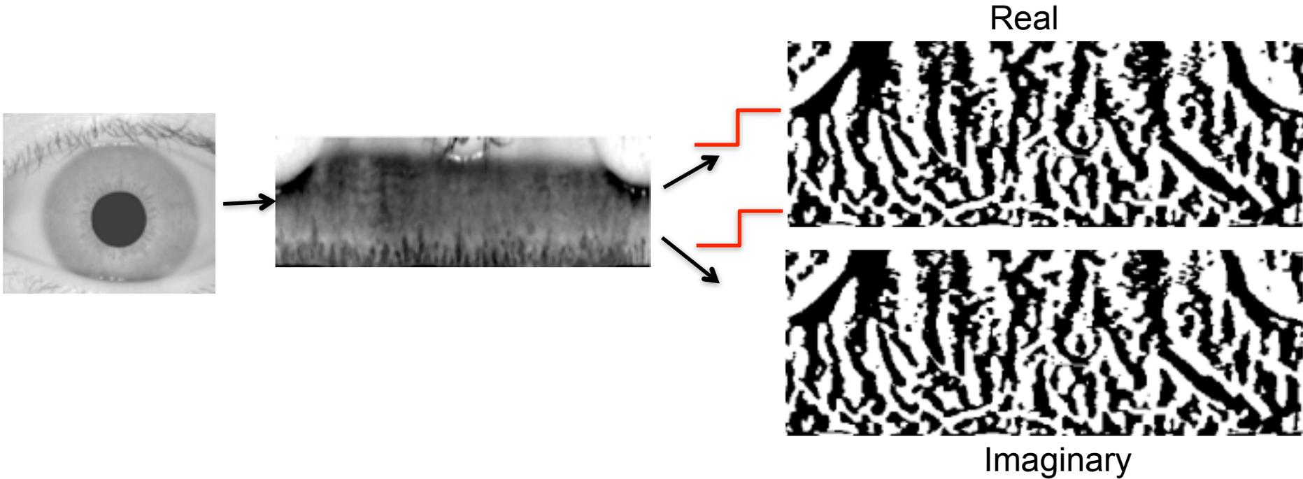
Iris codes are compared using Hamming distance
