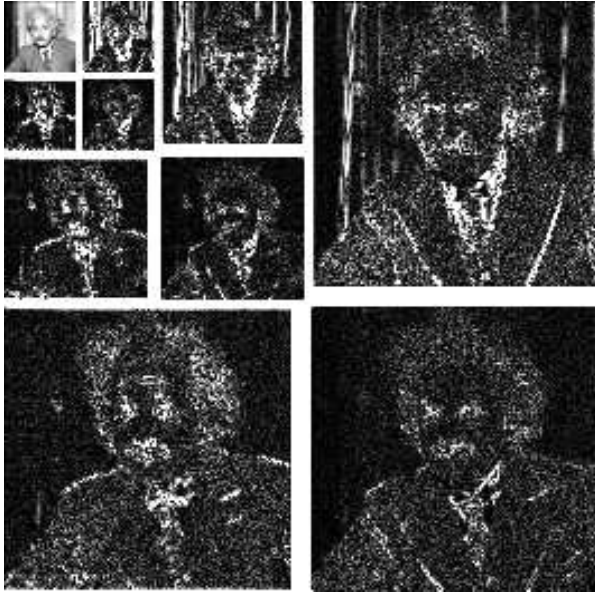
Fig. 7. Amplitudes of multi-scale wavelet coefficients for the “Einstein” image. Each subimage shows coefficient amplitudes of a subband obtained by convolution with a filter of a different scale and orientation, and subsampled by an appropriate factor. Coefficients that are spatially near each other within a band tend to have similar amplitudes. In addition, coefficients at different orientations or scales but in nearby (relative) spatial positions tend to have similar amplitudes.
