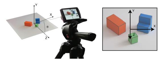
Figure 1.3: A simple projection model. a) world axis and camera plane. b) Visualization of the world axis projected into the camera plane with parallel projection. Note that the Z axis does not look like is pointing towards the observer. Instead, the Z axis is identical to the Y axis up to a sign change and a scaling. A point moving parallel to the Z axis will be indistinguishable from a point moving down parallel to the Y axis.
