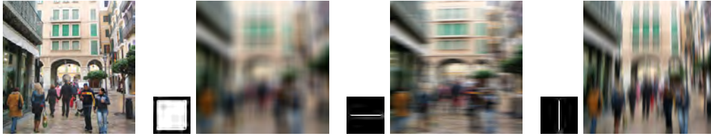
Figure 1.2: Blurring with a square, and a horizontal and vertical line. Note the structures that are both averaged out (along the direction of blurring), and maintained (perpendicular to that direction) in each resulting image.
