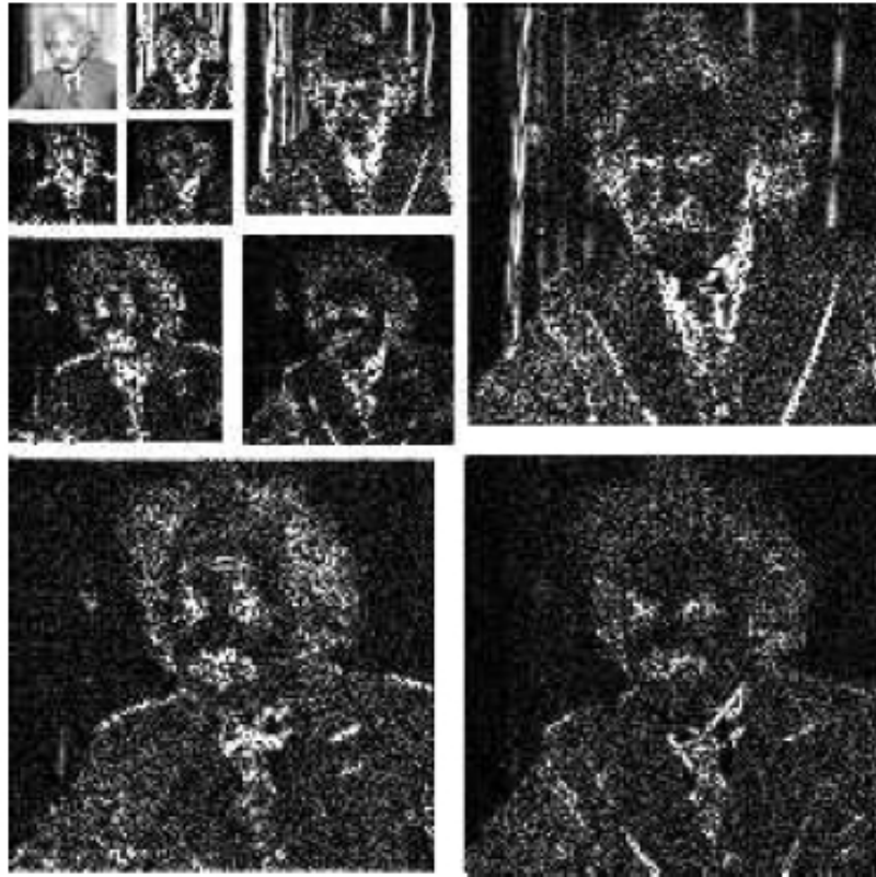
Fig. 7. Amplitudes of multi-scale wavelet coefficients for the "Einstein" image. Each subimage shows coefficient amplitudes of a subband obtained by convolution with a filter of a different scale and orientation, and subsampled by an appropriate factor. Coefficients that are spatially near each other within a band tend to have similar amplitudes. In addition, coefficients at different orientations or scales but in nearby (relative) spatial positions tend to have similar amplitudes.
